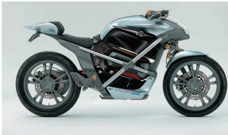
BATTERY BIKE: NEC TOKIN's Large-Size Mn Li-ion Laminate Battery was used in Suzuki's recent Crosscage prototype electric-powered motorcycle.
